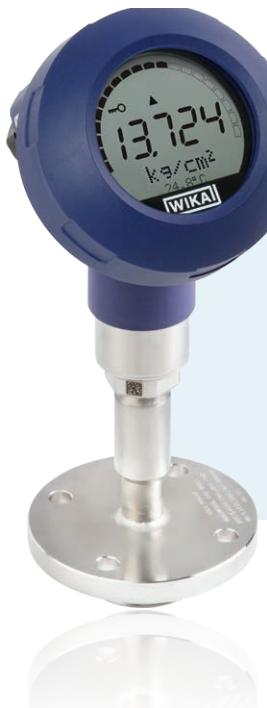
The in-line diaphragm seal is perfectly suited for use with flowing media. With the seal being completely integrated into the process line, measurements do not cause any disturbing turbulences, corners, dead spaces or other obstructions in the flow direction. The in-line diaphragm seal is clamped directly into the pipeline.
