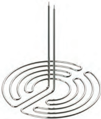
0.260 inch diameter, maximum heated length 118 inches based on minimum bend radius and cold end location
