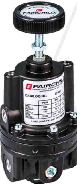
The Fairchild Model 15 Positive Bias Relay is designed for applications that require an output pressure that is the sum of a controlled input signal plus a fixed bias.
