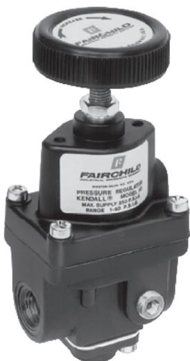
The Model 30 is designed for applications that require high capacity and accurate process control. A supply valve which is balanced by utilizing a rolling diaphragm, insures a constant output pressure even during wide supply pressure variations. Stability of regulated pressure is maintained under varying flow conditions through the use of an aspirator tube which adjusts the supply valve in accordance with the flow velocity.
