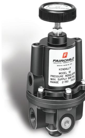
The Model 10 is designed for applications that require high capacity and accurate process control. A supply valve which is balanced by utilizing a rolling diaphragm, insures a constant output pressure even during wide supply pressure variations. Stability of regulated pressure is maintained under varying flow conditions through the use of an aspirator tube which adjusts the supply valve in accordance with the flow velocity.
