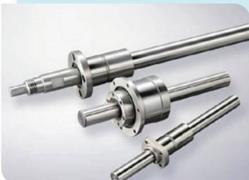
BALL SPLINE is linear motion rolling bearing with a round shaft having raceway grooves. It can be used in applications where torque transmission is required.
