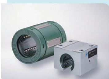
TOP BALL is linear motion rolling bearing with a round shaft, which is loaded by a plate with a raceway groove. It has greater load capacity compared to SLIDE BUSH, and has self-aligning feature.
