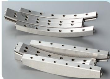
GONIO WAY is a curved cross roller slide way. It is a curved motion bearing utilizing low-friction, non-recirculating precision rollers. It is used when there is a need to change the gradient or obtain an accurate gradient angle without changing the center of rotation in high-precision optical and measurement equipment.
