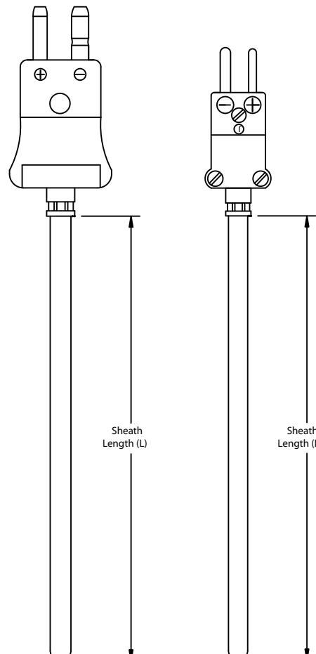
\*Note: GP thermocouples, manufactured using hollow tubing and wire, tend to be lower cost than MI, but cannot be bent in the field and are standardly designed for sensing temperatures below 500°F. MI thermocouples are more rugged than GP due to compacted magnesium-oxide powder insulation, can be bent in the field, and are appropriate for the temperature range of the sensor and sheath.
