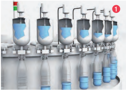
LEVEL MONITORING FOR BOTTLING BTL magnetostrictive linear position sensors
