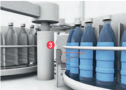
LABEL DETECTION ON BEVERAGE BOTTLES BOH Optical Sensor Heads
