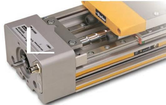
HMR belt driven actuators are designed for applications requiring high speed or long travel lengths. The belt driven version of the HMR gives OEM's the freedom to mount the motor in any of four positions at 90 degree intervals around the axis of motion, allowing the engineer to capitalize on space utilization and adding true value to the design process.
