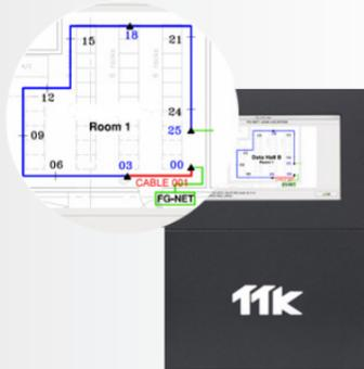
Dynamic map show the leak directly from the screen at real time
