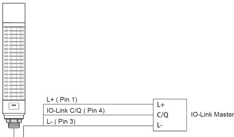
■ M12 Connector Pin Configuration
