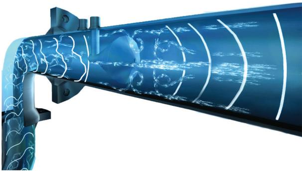
The contoured shape and location of the suspended cone in the V-Cone flow meter reshapes the velocity profile upstream. As the flow approaches the cone, the flow profile "flattens" toward the shape of a well-developed profile - even in extreme flow conditions.
