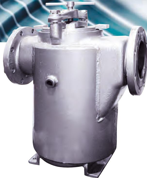
The Model 72SJ is for applications in which materials must be kept hot to remain fluid. Examples are chocolate, asphalt, resins and polymers. By circulating steam or a heat transfer fluid through the strainer jacket, the strainer body temperature remains constant.
