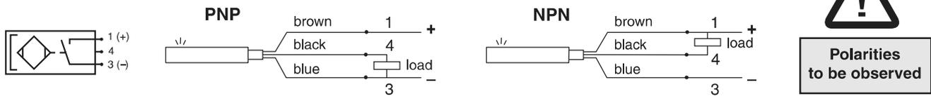
**CONNECTION OF MAGNETO-RESISTIVE DETECTORS: 3 possibilities**
